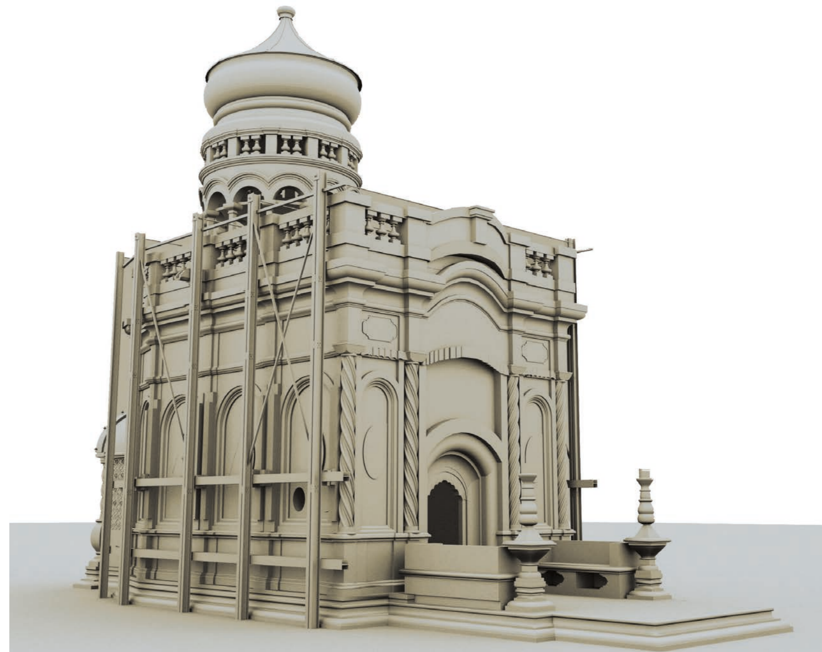
FIGURE 16 A view from the front of the Aedicula : the final model represents the architectural structure and the sustaining steel beams as well; only decorations as lamps and candles were disregarded.
